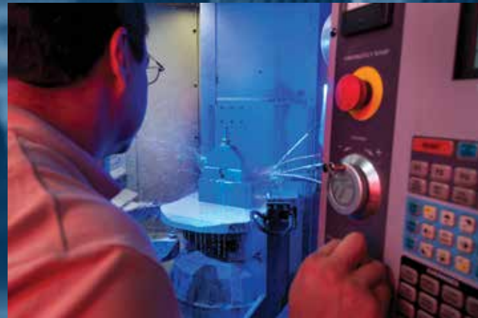
CNC programmer and machinist Gabe Bueno inspects cutting of pump blocks as they get machined using our Haas EC400 machining center.
